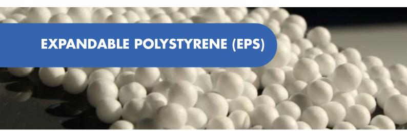
The expandable polystyrene (EPS) is a rigid cellular plastic with highly versatile uses, from medicine packages to construction industry and roads.
